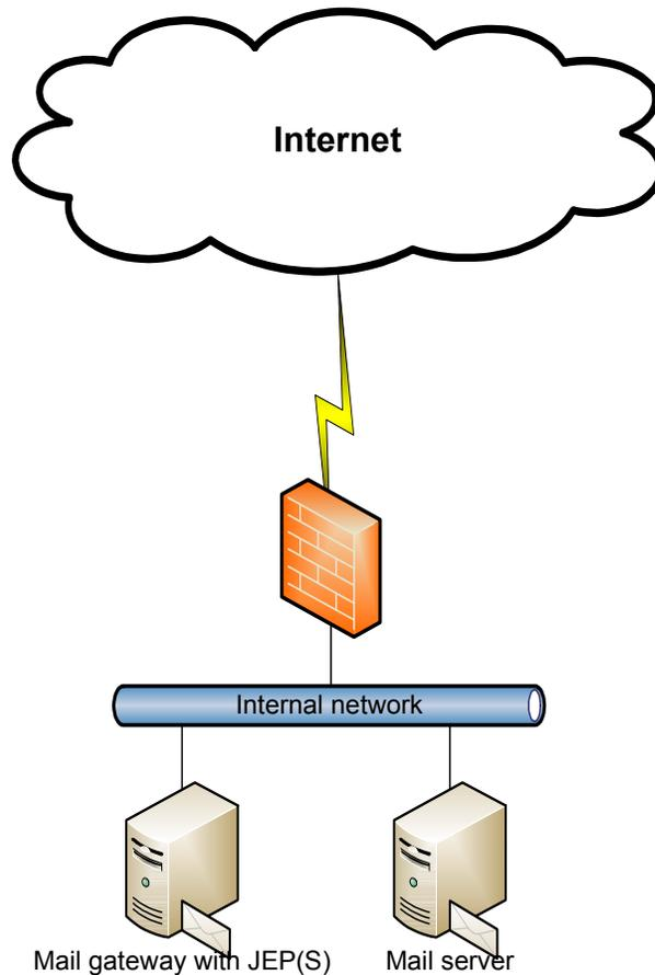
With this setup we achieve good security to a low cost. Both the JEP(S) Server and the JEP(S) sink are installed on the mail gateway. While its beneficial to place the mail gateway in a DMZ we do achieve a higher level of security and availability then with the single server setup.
