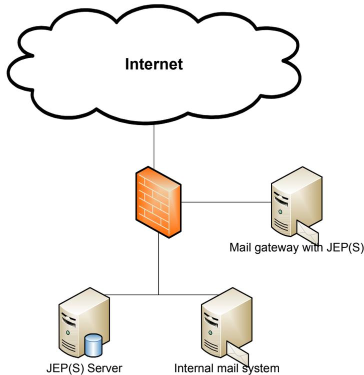
The above diagram explains the basics of setting up a security perimeter network. This is but one of the many different ways this can be setup and we'll go through many other scenarios later.
