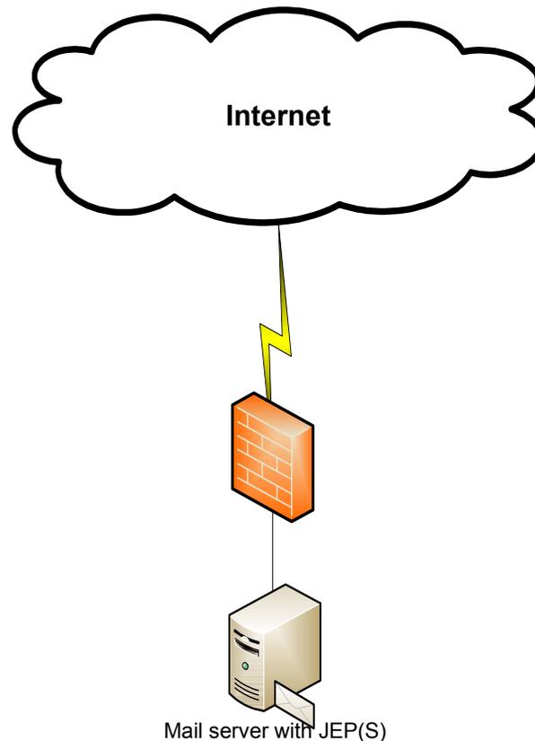
This is a common setup for small companies with Exchange, the JEP(S) server and the JEP(S) sink installed on the same server facing the internet. With a good firewall inspecting the SMTP packets the security achieved can be acceptable.
